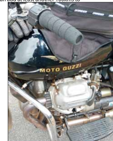
Below is a close up of Daniel's 1976 Moto Guzzi Convert 1000. If you look closely there is not clutch lever, cable or gear stick. Complete automatic transmission, just open the throttle and go!!! These bikes were popular with the Italian Police as escort bikes.
